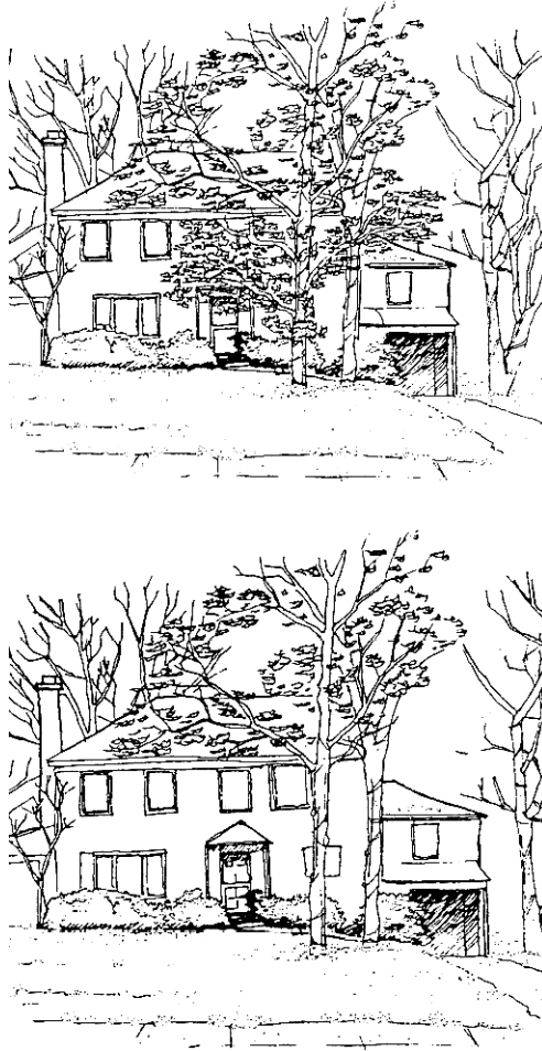
Figure A.6. Trees south of a home before and after pruning. Lower branches are pruned up to increase heat gain from winter sun (Sand 1993).
