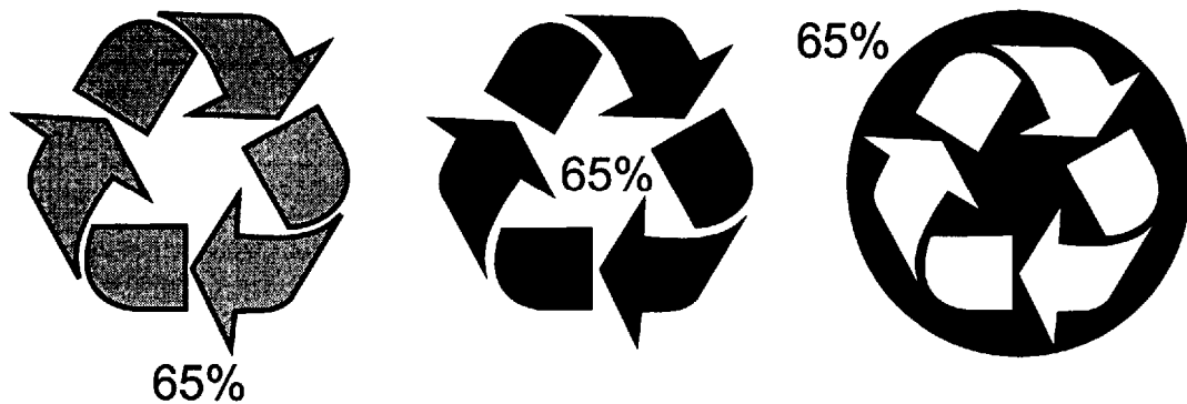
Figure 2 — Examples of acceptable locations of percentage value when using the Mobius loop to make claims about recycled content
